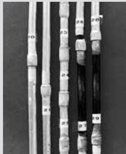
Figure 5, Tubes after pulsation tension test
