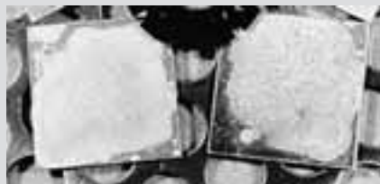
Figure 3, Appearance of flux residues after test cycle
