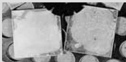
Figure 2, Appearance of flux residues before test cycle
