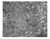
The aluminum coupons (AA3003 with 4343 clad) were fluxed with loads ranging from 3 to 7 g/m<sup>2</sup>. All samples were subjected to a standard cycle under CAB conditions with maximum temperature at 600 °C. The coupons were placed in the furnace without an aluminum angle. After cooling, they were collected, weighted and placed in the SWAAT chamber for a test with an acetic acid/sodium chloride solution.
