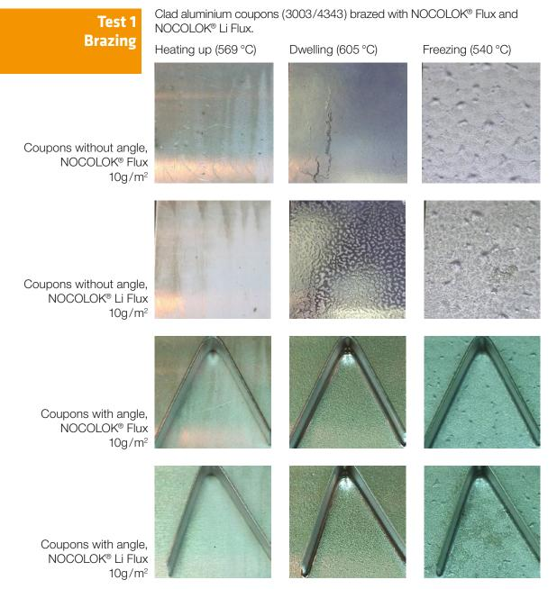
Notice that the breakup of the oxide layer at 605  $^\circ \rm C$  seems to be more efficient with NOCOLOK  $^{\rm \tiny II}$  Li Flux.
