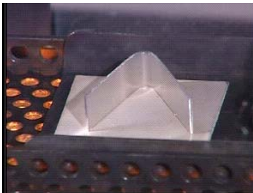
Picture 2: Angle-on-coupon test with binder spray application of NOCOLOK® Flux – During heat-up
