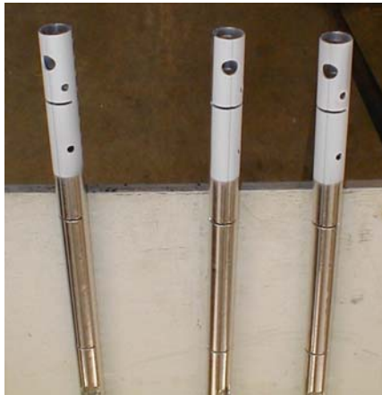
Picture 6 and 7: Selectively pre-fluxed condenser headers – NOCOLOK® binder spray application
