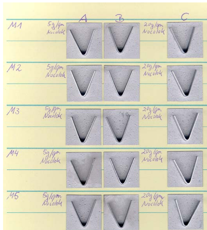
Picture 4: Angle-on-coupon tests with binder spray application of NOCOLOK® Flux A and B: 5g/m 2 flux load C: 20g/m 2 flux load M 1 – M 5: different binder mixtures
