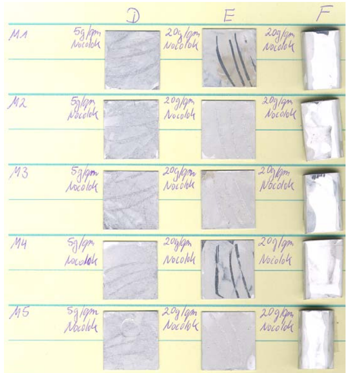
Picture 5: Aluminum-coupons coated with binder-based NOCOLOK® Flux slurry D: 5g/m 2 flux load E and F: 20g/m 2 flux load M 1 – M 5: different binder mixtures Column F shows coupons after bending
