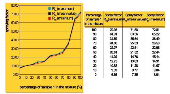
The ability of a powder to fluidize is very important for its performance in electrostatic application. However, it is not the only factor.
