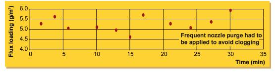
These results were confirmed by other observations made during additional trials. Material with spray factors of approximately 45 g/0.5 min and higher (with good fluidization) flowed through the equipment pipes and hoses with less material buildup and created lower amounts of residue buildup on the spray nozzles.
