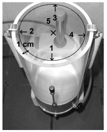
Indication of the locations for the measure of the height of the powder in both fluidized and non fluidized condition.
